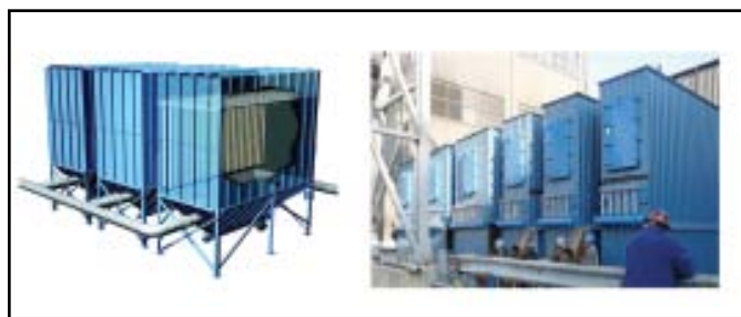
Figure 3. Multiple housing modules are operated in parallel to handle large volumetric flow rates.
