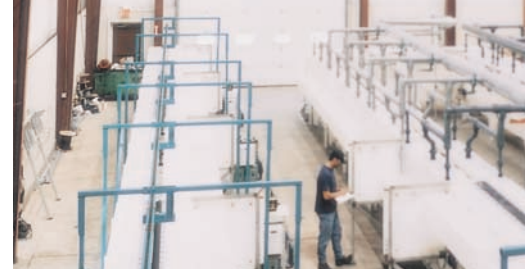
Complete washer assembly showing conveyor, recirculation pump subassemblies and multi-station format.
