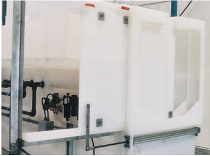
Automatic actuating polypropylene door assembly designed to separate wash system chemistry.
