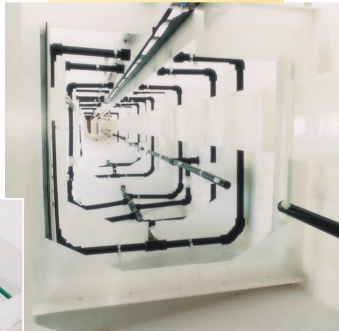
► Internal view of all-polypropylene acid etch wash/ rinse stations.
