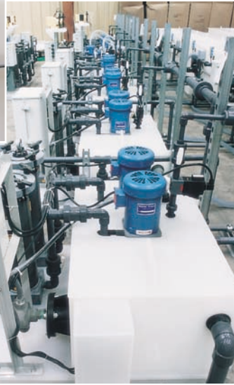
▲ Detail showing dual pump washer tanks with connecting pumping systems.
