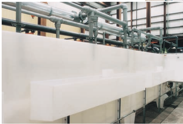
Polypropylene washer assembly showing partial piping and ventilation pickup points.
